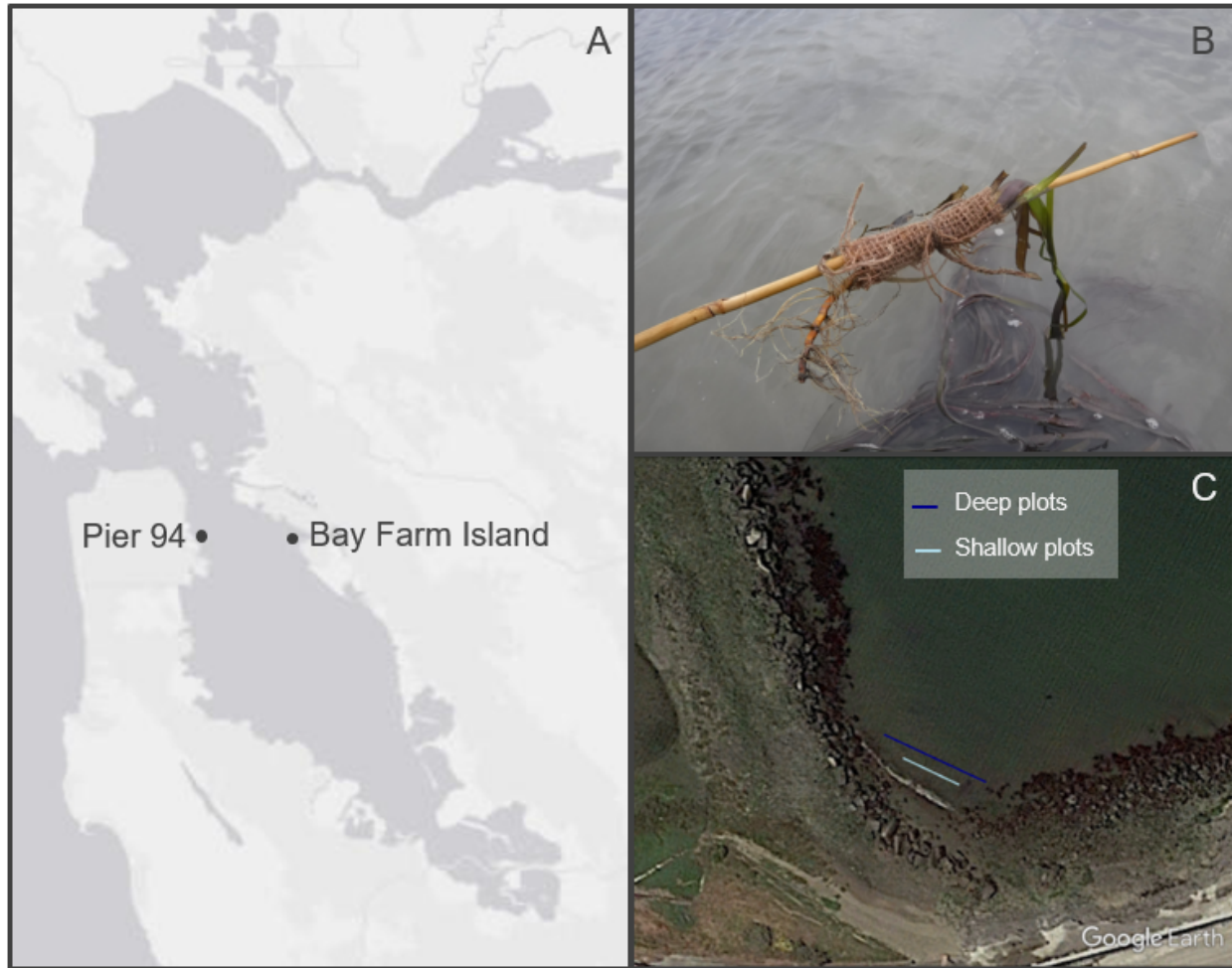
Figure 1. A) Map of Pier 94 (study site) and Bay Farm Island (eelgrass donor site) in San Francisco Bay; B) eelgrass transplanting unit; C) Satellite image showing locations of the shallow (-1.5 ft MLLW) and deep (-2 ft MLLW) plots at Pier 94.
