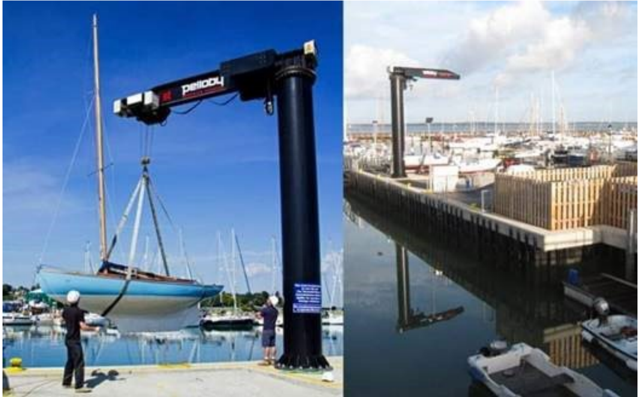
Figure 5. Example of jib boom crane / boat hoist setup (Source: Pelloby Cranes)
